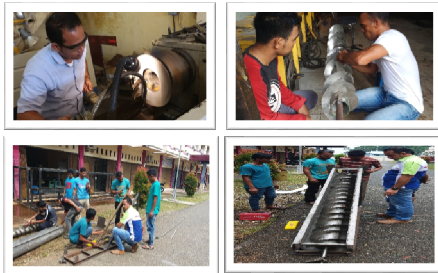
Figure 6. Fabrication Archimedes Single Screw Turbine
