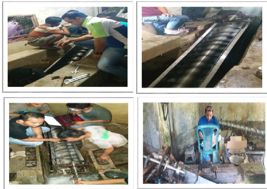
Figure 7. Activities for Testing and Collecting Performance Data Archimedes Single Screw
