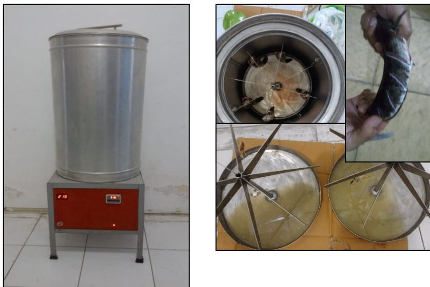
Fig 5. The final design of the snakehead fish ( Channa striata ) extraction prototype
