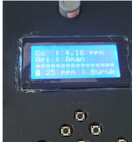
Fig. 6. MQ7 sensor reading results at gas levels of 4.16 Ppm
