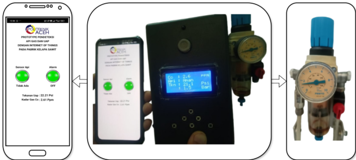
Fig. 9. Display of vapor pressure on LCD and smartphone
