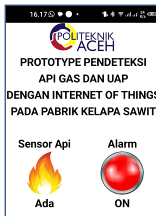
Fig. 11. Smartphone screenshot for alarm testing when fire is detected
