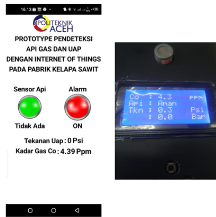
Fig. 13. Alarm testing with gas levels exceeding 3 PPM.
