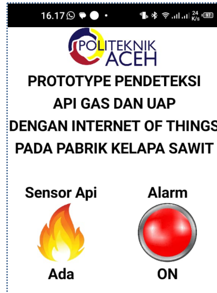
Fig. 8. Display of the detected Fire sensor on the smartphone
