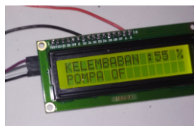
Fig 5. Soil Moisture 55% and Water Pump Off
