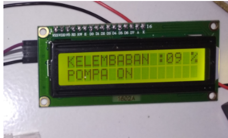
Fig 3. Humidity 9% and Water Pump On
