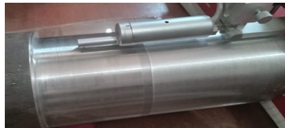
Fig 9. Surface roughness value at cutting condition 2 ( v = 62 m/min; a = 1 mm; t_c = 5.29 min)
