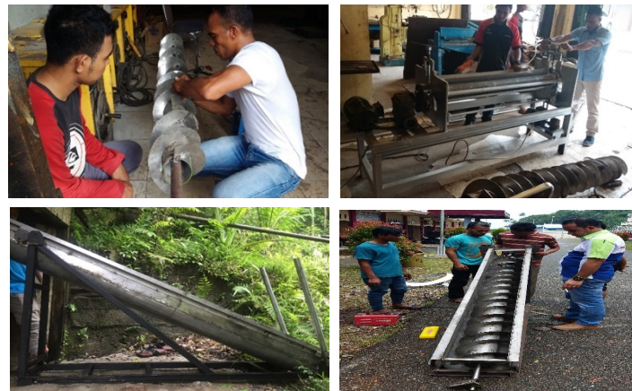
Fig. 7. Manufacture Archimedes Double Screw Turbine
