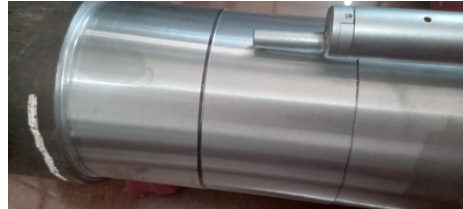
Fig. 10. Surface roughness value at cutting condition 2 ( v=235 m/min| f=0.75 mm/put| a=1 mm| t_c=5.30 min)
