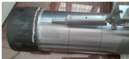
Fig. 11. Surface roughness value at cutting condition 3 ( v=235 m/min| f=0.1 mm/put| a=1.5 mm| t_c=5.45 min)
