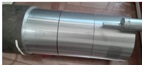
Fig. 9. Surface roughness value at cutting condition 1 (v= 235 m/min|f= 0.05 mm/put|a=0.5 mm|t c = 5.23 min)
