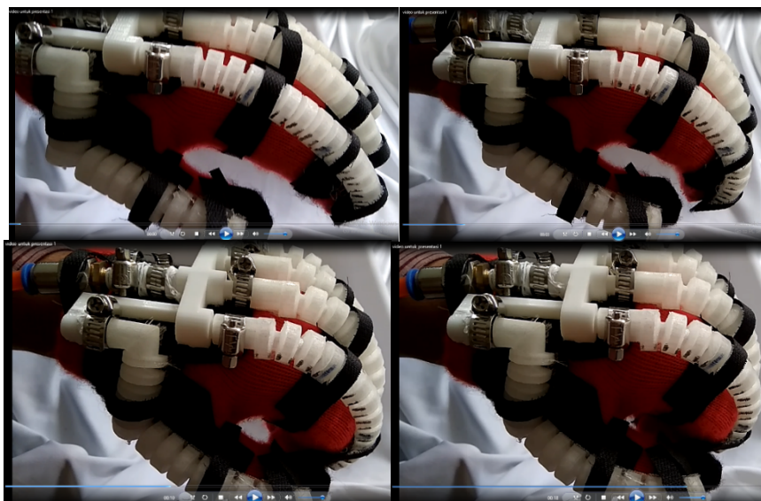
Fig. 6. Applying M3 with the glove to move human hand in grasping movement.
