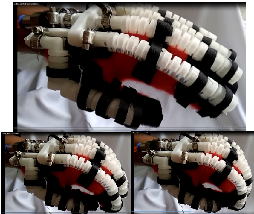
Fig. 5. Applying M3 with the glove to move human hand in picking-like movement.
