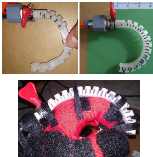
Fig. 3. The SPAs were inflated and measured. A. Unloaded M1. B. Unloaded M2 C. The loaded SPA. [18]
