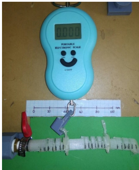
Fig. 4. The measurement of force generated by each joint of SPA.[18]
