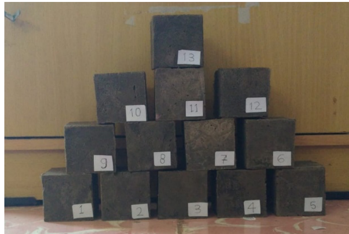
Fig. 1. The hardened geopolymer, a result of mixing according to the RSM method
