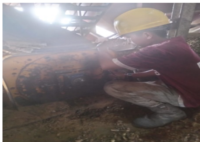
Fig. 3. Ripple mill machine rotor axle inspection process
